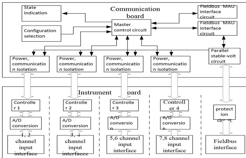
Figure 3.1 Hardware diagram of smart temperature transmitter
