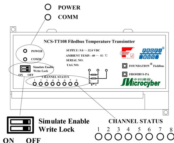
Figure 4.4 DIP switch of NCS-TT108 Smart Temperature Transmitter
